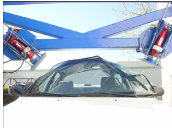
Figure 3. M216 two-sided static test machine.
