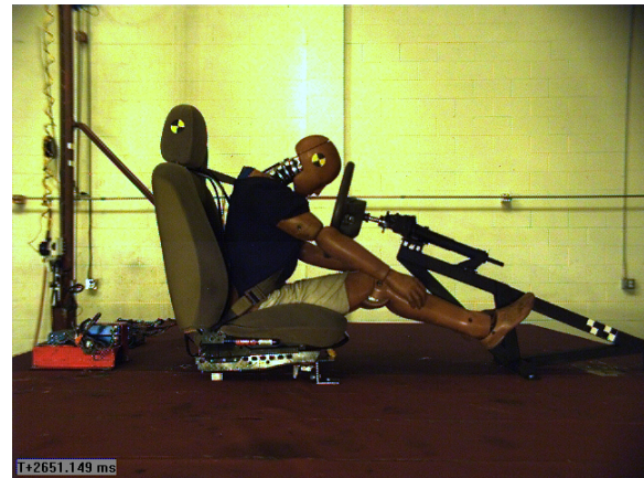
Figure 25. Hybrid III dummy with original musculature neck.
