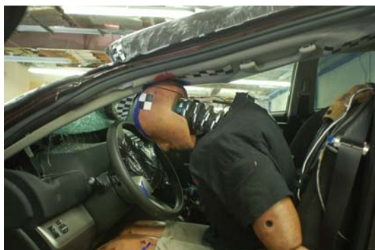
Figure 12. Soft neck of hybrid III dummy.
